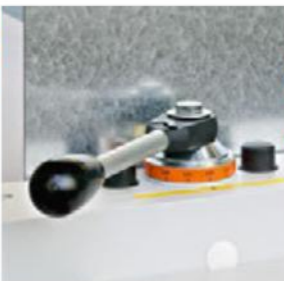
Cutting gap setting can be adjusted without tools
