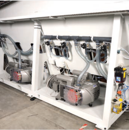
Vacuum pumps integrated in the machine frame
