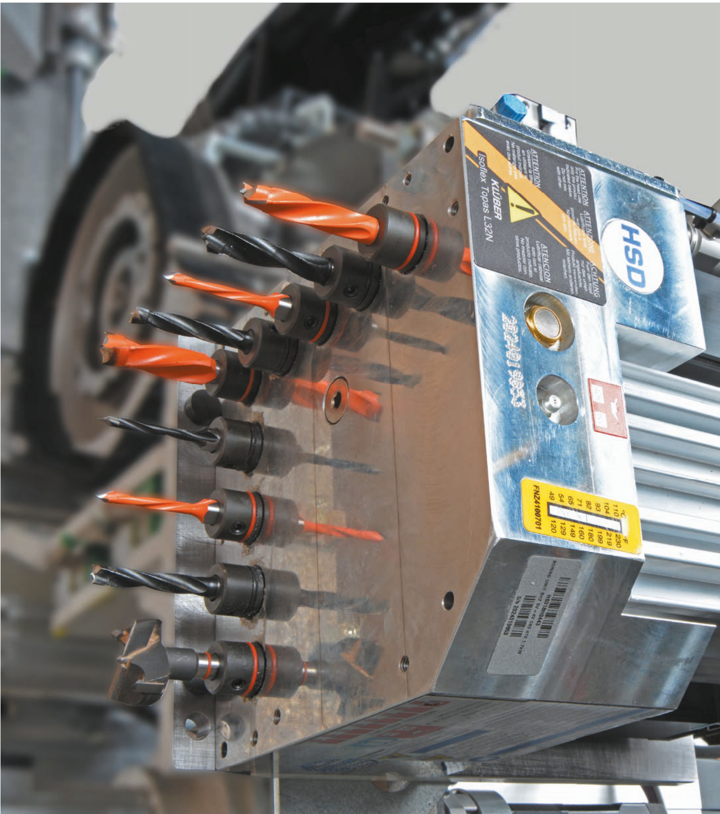
9 spindle drilling unit
