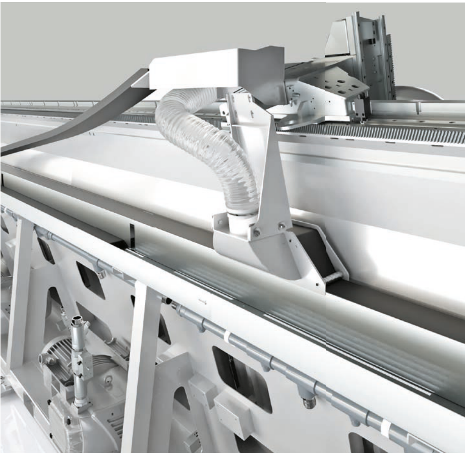
Vacuum channel along the entire length of the X-axis for optimised chip collection
