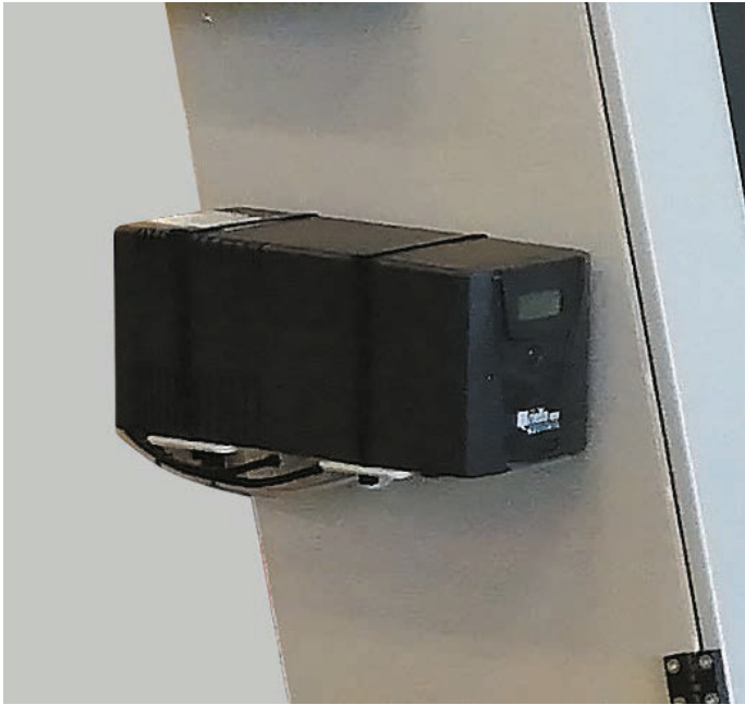
Electric back-up UPS for PC protection and power supply
