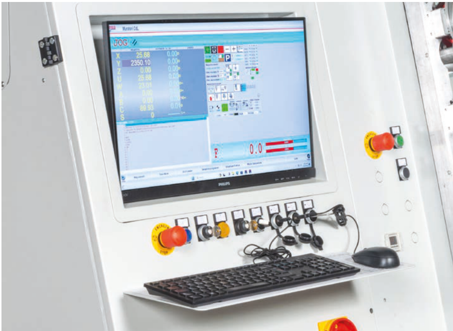
PC integrated in the electrical cabinet, with 24" protected and tiltable screen
