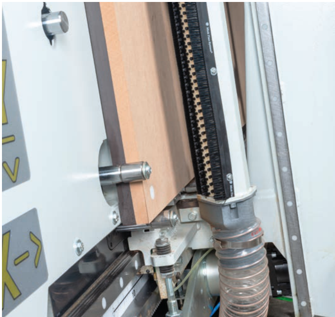
Motorised brush for cleaning the worktable, with dust extraction
